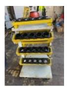
Tooling cart for 50 taper tooling on wheels
